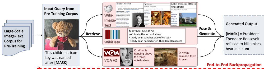
Figure 1. We augment a visual-language model with the ability to retrieve multiple knowledge entries from a diverse set of knowledge sources, which helps generation. Both retriever and generator are trained jointly, end-to-end, by optimizing a language modeling objective.
